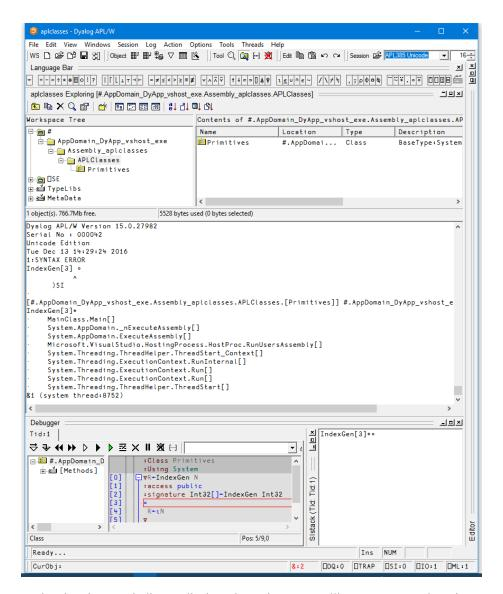
Notice that the state indicator displays the entire .NET calling structure, and not just the APL stack. In this case, the state indicator shows that IndexGen was called from MainClass.Main, which combines the class and method names specified in aplfns.cs. Note that .NET calls are slightly indented.
